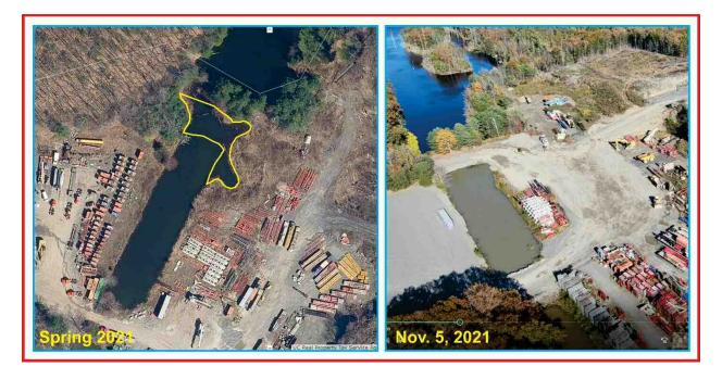
Figure 7. Unpermitted dam construction and blockage of Pickerel Pond outflow within the headwaters of Praymaher Brook. The yellow polygon approximates a 0.3-acre fill zone. Drone imagery documents fill placement sometime between 9-30-21 and 11-05-21.
