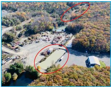
Figure 4. Sediment laden Pond B exhibits the uncontrolled release of fine particulates into Praymaher Brook.
